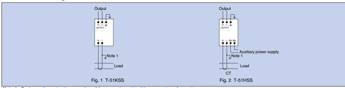
Note 1. For low-voltage circuits, grounding of the secondary side of the current transformer is unnecessary.
