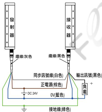
Receiver(RX) PNP output circuit diagram
