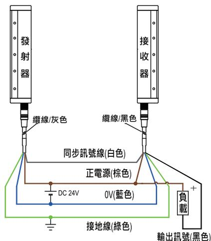
Receiver(RX) NPN output circuit diagram
