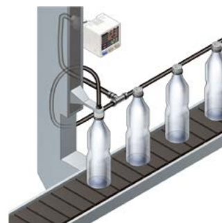
Air-leak test for PET bottles
