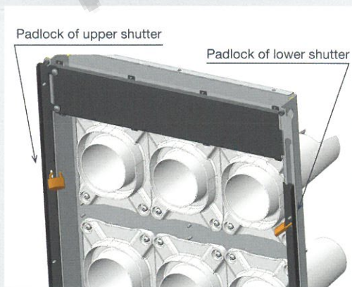
The shutter is open position
