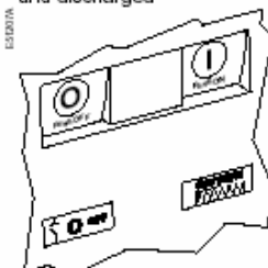
Circuit breaker open and discharged
