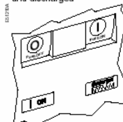
Circuit breaker closed and discharged
